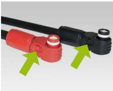
When installing the DC cabling, please note the following: **The plugs must audibly click into place.** The plugs can be unlocked by pressing the pushbutton on the side of the plug (see markings in the illustration).
