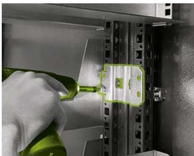
Then fasten the middle and the top cabinet baying connectors using the front holes and four screws (H.2). Then refit the relevant slide rail.
