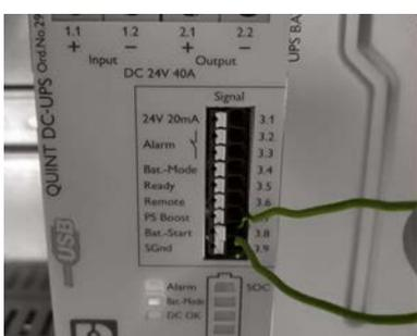
Perform a cold start of the UPS 93. With the cold start function, the UPS can be started without an input supply voltage. The UPS is powered by energy from the connected battery, which also supplies the loads. The two signal terminals Bat.-Start (3.8) and SGnd (3.9) must be connected briefly. After initialisation, the UPS switches to battery mode.
