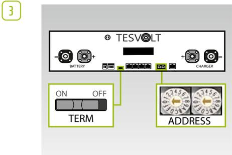
Check and, if necessary, correct the settings for terminating and addressing the TS HV80 "TERM" 5 and "ADDRESS" 10 on the APU HV1000-S.
