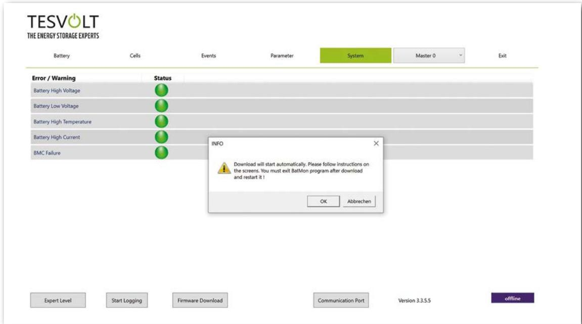
The latest firmware can then be downloaded with the "Firmware download" button on the "System" tab.
