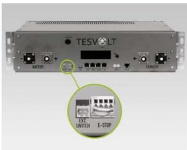
The four-pin plug for the e-stop connection on the APU HV1000-S must be plugged in for operation. The APU HV1000-S will remain inactive without this plug. Further information about the e-stop can be found in the section "8.3 E-stop contact" on page 45.
