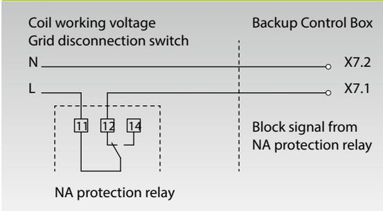
**X8 Control of the coil of the grid isolator**
