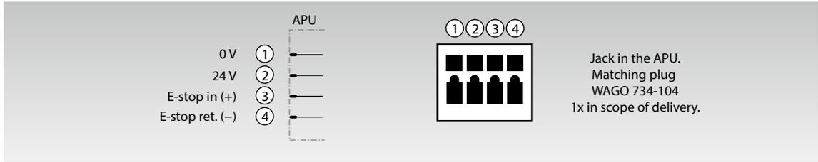
Figure 8.2 Assignment of the e-stop connection jack 4
