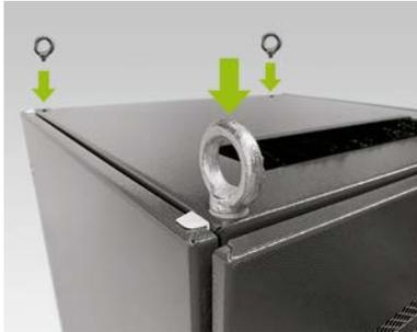
**Optional: Install the ring screws:** Install four ring screws at the four corners of the cabinet halves to transport the individual halves of the cabinet by crane. To do this, remove all the fastening screws from the cabinet covers and replace them with the ring screws (L).
