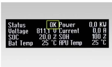
After precharge mode, the on/off "SWITCH" 17 stays lit. "OK" appears as the status on the display of the APU HV1000-S. The TS HV80 is now ready for operation.
