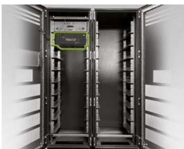
Insert the first battery module into the slide rails below the APU HV1000-S. Affix it to the pre-fitted cage nuts using four M6 x 16 pan head screws (1) (cross-head) incl. plastic washers (1.1). Now fit the remaining modules in the left half of the cabinet.
