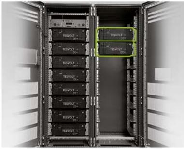
As soon as the left half of the cabinet has been filled, install the battery modules in the right side. Start at the level of the top left module (the position at a level with the APU HV1000-S remains unoccupied). Affix the module to the pre-fitted cage nuts (J) with four M6 x 16 pan head screws (I) incl. washers (II). Then, place the next module below the one that has already been installed and fasten it as described. Continue until all the modules have been installed.
