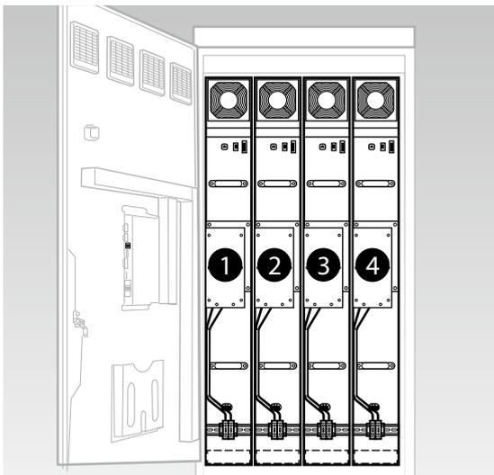
The installation position of the IPU determines the assignment of the associated NH isolators and circuit breakers. An overview is given in the following table.
