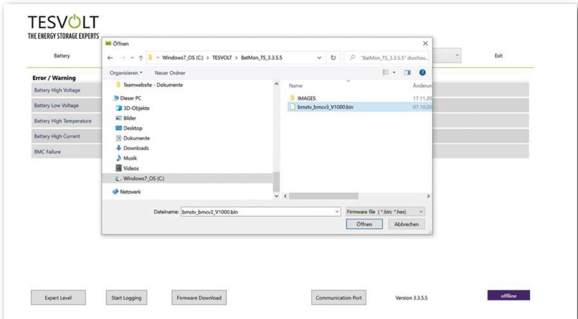
In the window that opens, select the firmware file (.bin) and confirm the selection by clicking on "Open".
