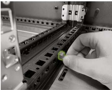
Fit the cabinet grounding connection set (M) to equalize the potential between the two halves of the cabinet. To do this, insert the speed nuts (M5) from the side into the two middle cabinet profiles at the cabinet base. You are free to choose the position, but both speed nuts must be directly opposite each other.
