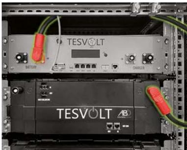
The battery modules on the TS HV80 are interconnected in series. The colours of the plugs must match the colours of the jacks on the battery module, i.e. red plug to red jack, for example. Start on the left side of the cabinet with the APU HV1000-S and the first battery module with the connecting cable (3.1).
