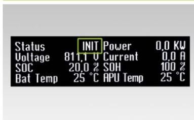
The TS HV80 switches to "INIT" mode and the on/off "SWITCH" 17 starts to flash.
