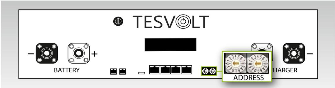
Set the address selector on the APU HV1000-S to match the configuration and data in the table below.
