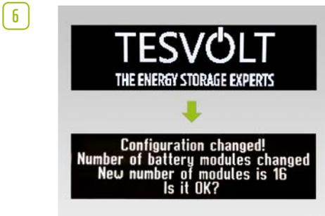
The number of detected battery modules (16) is shown on the display. Confirm the correct number by tapping twice on the marking 16 next to the display. If the displayed number of modules differs from the number actually present, shut down the device and check the BAT-COM wiring. If the fault continues to occur regardless, please contact the TESVOLT Service Line +49 (0) 3491 8797-200 or via email to [service@tesvolt.com](mailto:service@tesvolt.com).
