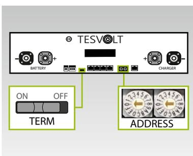
Now you can make the settings for terminating and addressing the TS HV80 "TERM" 5 and "ADDRESS" 10 in accordance with section "Overview of all addressing options" on page 87 et. seq. In the case of master/slave systems, TERM 5 is to be set to "ON" for the APU HV1000-S of the master and the last storage system in the master/slave configuration. TERM 5 is to be set to "OFF" for all other slave APUs in the configuration.
