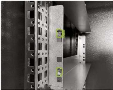
Now, fit the cage nuts (J) for fastening the battery modules (2) with the auxiliary tool (J1) (see "5.8 Wiring the battery modules" on page 24 for the positions of the battery modules). Distribute the cage nuts from bottom to top. Start at the bottom edge of the slide rail for the relevant battery module. Fit the first two cage nuts in the second opening on both sides from below, and fit the remaining two cage nuts in the top opening in the two slide rails.
