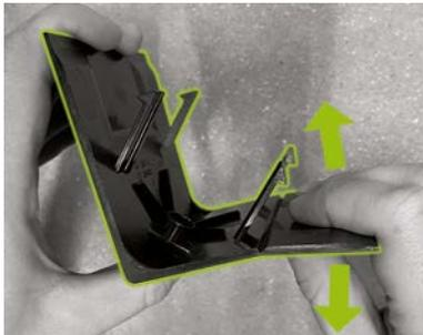
Prepare a right base corner cover plate (G) (with the logo on the left leg) for fitting on the cabinet base. To do this, break the cover plate in half at the notch on the right leg. The narrow piece can be disposed of. Now use the two hooks of the connector for the base corner cover plate (G.2) to attach it to the shortened cover plate's short leg.
