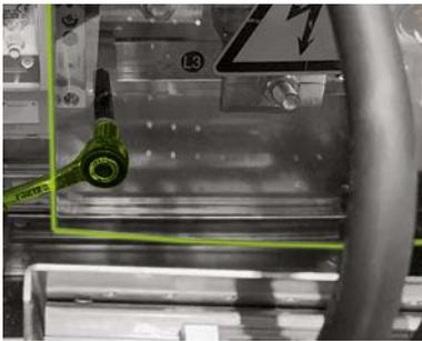
Now remove the touch guard above the AC connections (26). To do this, loosen the two M6 screws and remove the touch guard.
