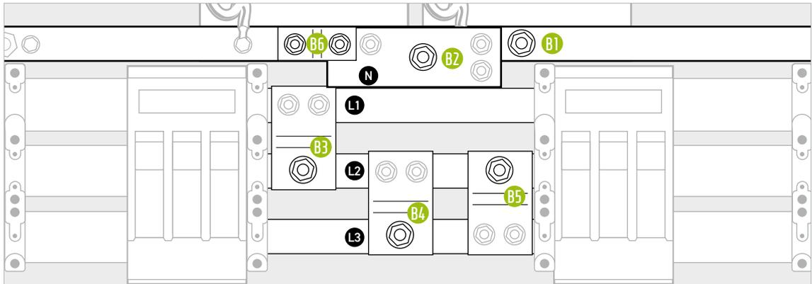
Figure 9.2 AC connector panel (behind the DC connections)
