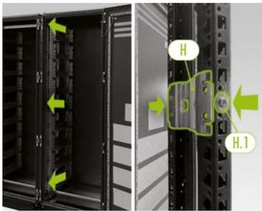
First of all, on the front of the cabinet, attach three baying connectors (H) to the central vertical cabinet profiles inside the cabinet at the top, middle and bottom. The baying connectors are affixed to the frame profiles with two setscrews (H.1) on each side from the right and left.
