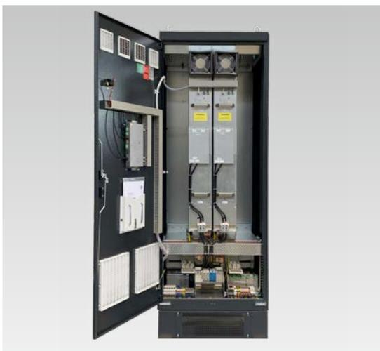
The battery storage system TESVOLT TS-IHV80 is equipped with the three-phase battery inverter TESVOLT PCS. It has a modular design and can be equipped with up to four inverter modules with 75 kW each.
