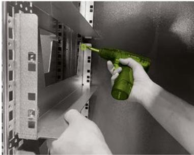
Now, fit the remaining three baying connectors (H) to the cabinet profiles at the rear of the cabinet at the same height as the front baying connectors already installed. When fitting the bottom baying connector, use the same process as for fitting on the front cabinet profiles. However, for the top and middle cabinet baying connectors, you must first remove the slide rail on one side in the fitting area.
