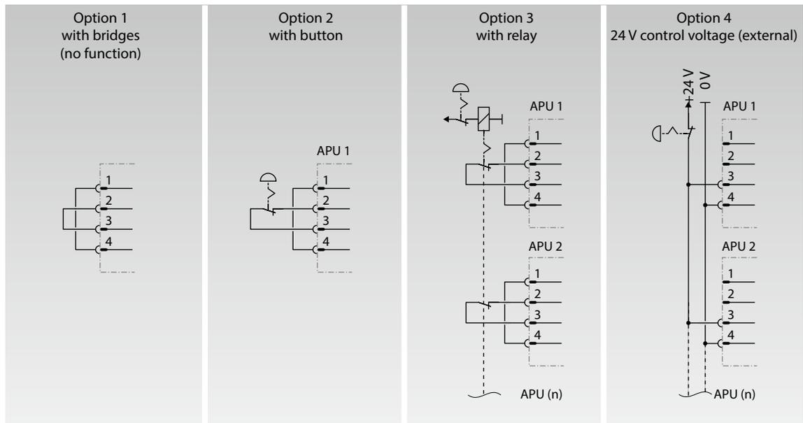
Figure 8.1 Different wiring options for the e-stop; options 3 and 4 are intended for use in systems with more than one APU HV1000-S.
