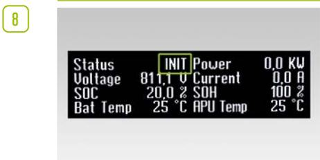
TS HV80 switches to "INIT" mode and the on/off "SWITCH" 17 starts to flash.
