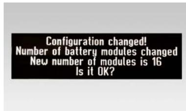
The display of the master APU HV1000-S now shows the number of detected battery modules (16). Confirm the correct number by tapping twice. In case of deviations, shut down the TS HV80 and check the BAT-COM cabling. If the fault continues to occur regardless, please contact [service@tesvolt.com](mailto:service@tesvolt.com) or the TESVOLT Service Line +49 (0) 3491 87 97 - 200.
