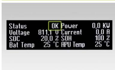
Once the precharging has completed successfully, the on/off switches "SWITCH" 17 on all APU HV1000-Ss in the master/slave configuration are permanently illuminated. "OK" appears as the status on the display of the APU HV1000-S. All the TS HV80 units are now ready for operation.
