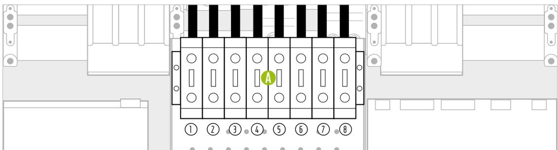
Figure 9.1 DC connector panel (covers the AC connection)
