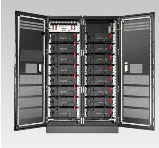
The battery storage system TESVOLT TS-IHV 80 is equipped with the high-voltage lithium battery storage TS HV 80. The battery storage is modular and has 16 battery modules with a capacity of 4.8 kWh each.
