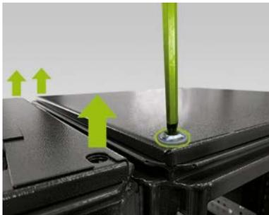
**Optional: Installing the combined brackets:** If you would like to transport the assembled cabinet (without the battery modules) by crane, two combined brackets (0) have to be fitted. To do this, remove the two fastening screws from the cabinet covers on each side of the two halves of the cabinet that are connected to one another (four screws in total).
