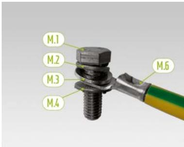
Now prepare the grounding cable (M.6) for installation. To do this, put an M8 spring washer (M.2), an M8 washer (M.3), the grounding cable's cable eyelet (M.6) and finally the M8 contact washer (M.4) onto the M8 screw (M.1). Ensure that the teeth of the M8 contact washer (M.4) are pointing downwards, towards the end of the screw.
