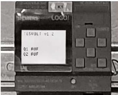
The control program for the Siemens Logo (K1) <sup>92</sup> is already implemented in the factory configuration (recognisable by the display of "TESVOLT v1.2"). The display also indicates that both grid isolators are open ("Q1 OPEN"; "Q2 OPEN").
